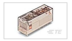
Power Relay Type: Force-Guided Coil Magnetic System: Monostable, DC Coil Power Rating Class: 800 – 1000 mW Coil Power Rating DC: 800 mW Coil Resistance: 180 Ω
